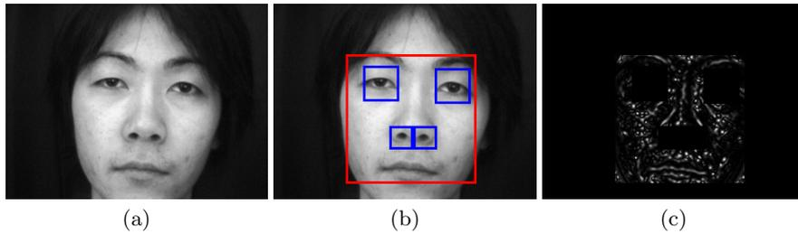
**Fig. 7.** Pre-processing for generating the shape subspace: (a) input image, (b) detected face, pupils and nostrils, (c) separability map.
