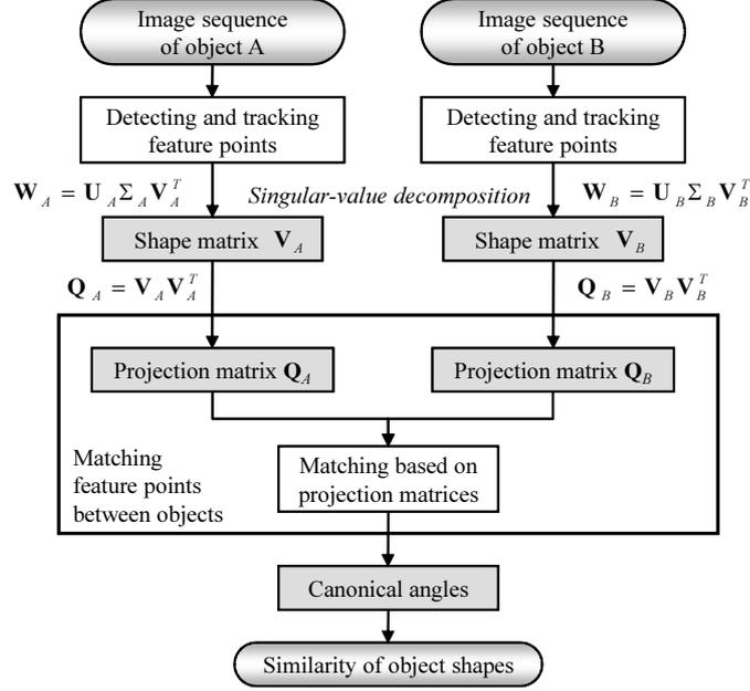
Fig. 4. Flow of the object recognition process based on the proposed similarity measure.
