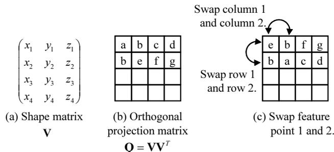
**Fig. 2.** Example of swapping rows and columns of the orthogonal projection matrix by swapping feature points. ( $P = 4$ )
