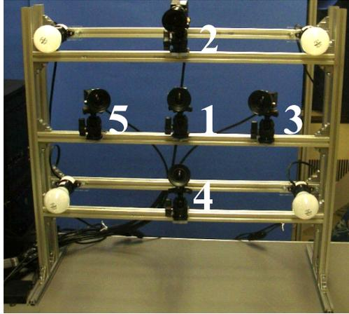
**Fig. 4.** Multiple-camera system.
