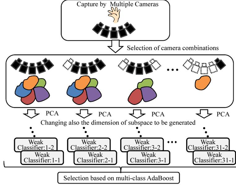
**Fig. 2.** Conceptual diagram of proposed method: Various weak classifiers are generated by changing the combinations of the cameras used for recognition and the dimensions of reference subspaces. Valid weak classifiers are selected using multi-class AdaBoost learning.
