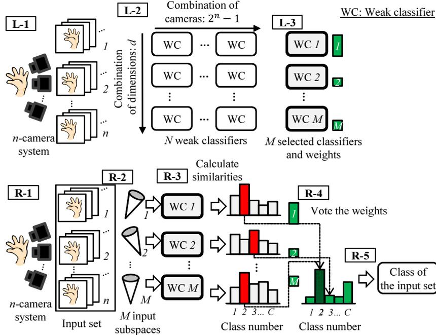
Fig. 3. The flow of the hand shape recognition process based on the proposed method.
