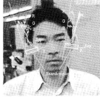
図3 顔輪郭付近における RGB 輝度・分離度の分布 Fig.3 Profiles of image intensity of RGB and separability near a face contour.
