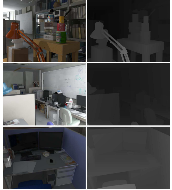
Figure 5: Some example frames from the dataset with their respective depth maps obtained by applying a custom ramp shader to the geometry of the scene.
